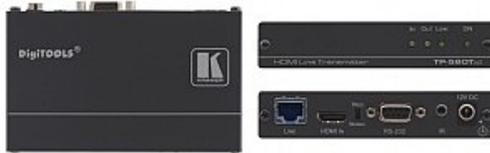
TP-580Txr is a high-performance, extended-reach HDBaseT transmitter for 4K60Hz (4:2:0) HDMI, RS-232 and IR signals over twisted pair. The TP-580Txr converts all input signals into the transmitted HDBaseT signal. It extends video signals to up to 100m (330ft) over CAT copper cables at up to 4K@60Hz (4:2:0) 24bpp video resolution and provides even further reach for lower HD video resolutions
